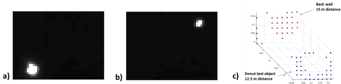
Fig. 3. a) Image of light emitted from grating switch when the first switch in the path is on, and b) when the 70 th switch in the path is on. Even at this high gain setting, with the camera clearly saturating, there is no background visible on this scale. c) LiDAR data of donut test object and the wall beyond it. The field of view is approximately 1°.
